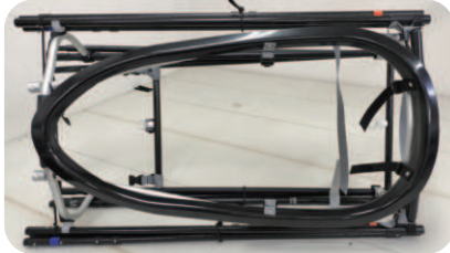
① Remove all parts from the backpack ② Install gunwales and keel frame ③ Attach bow, stern and rib frames ④ Insert the frame into the hull skin
