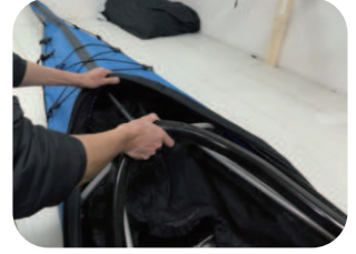
① Remove all parts from the backpack ② Install gunwales and keel frame ③ Attach bow, stern and rib frames ④ Insert the frame into the hull skin
