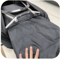
① Remove all parts from the backpack ② Install gunwales and keel frame ③ Attach bow, stern and rib frames ④ Insert the frame into the hull skin
