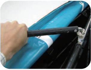
⑤ Apply hull tension with the built-in winch ⑥ Close and secure the stern section ⑦ Inflate the side air tubes ⑧ Install the seat and complete assembly
