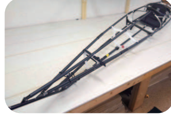
① Remove all parts from the backpack ② Install gunwales and keel frame ③ Attach bow, stern and rib frames ④ Insert the frame into the hull skin
