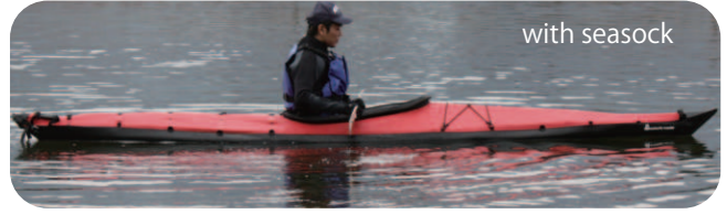
Fully flooded cockpit condition
