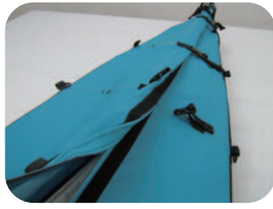
⑤ Apply hull tension with the built-in winch ⑥ Close and secure the stern section ⑦ Inflate the side air tubes ⑧ Install the seat and complete assembly
