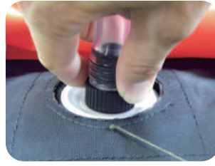
⑤ Apply hull tension with the built-in winch ⑥ Close and secure the stern section ⑦ Inflate the side air tubes ⑧ Install the seat and complete assembly
